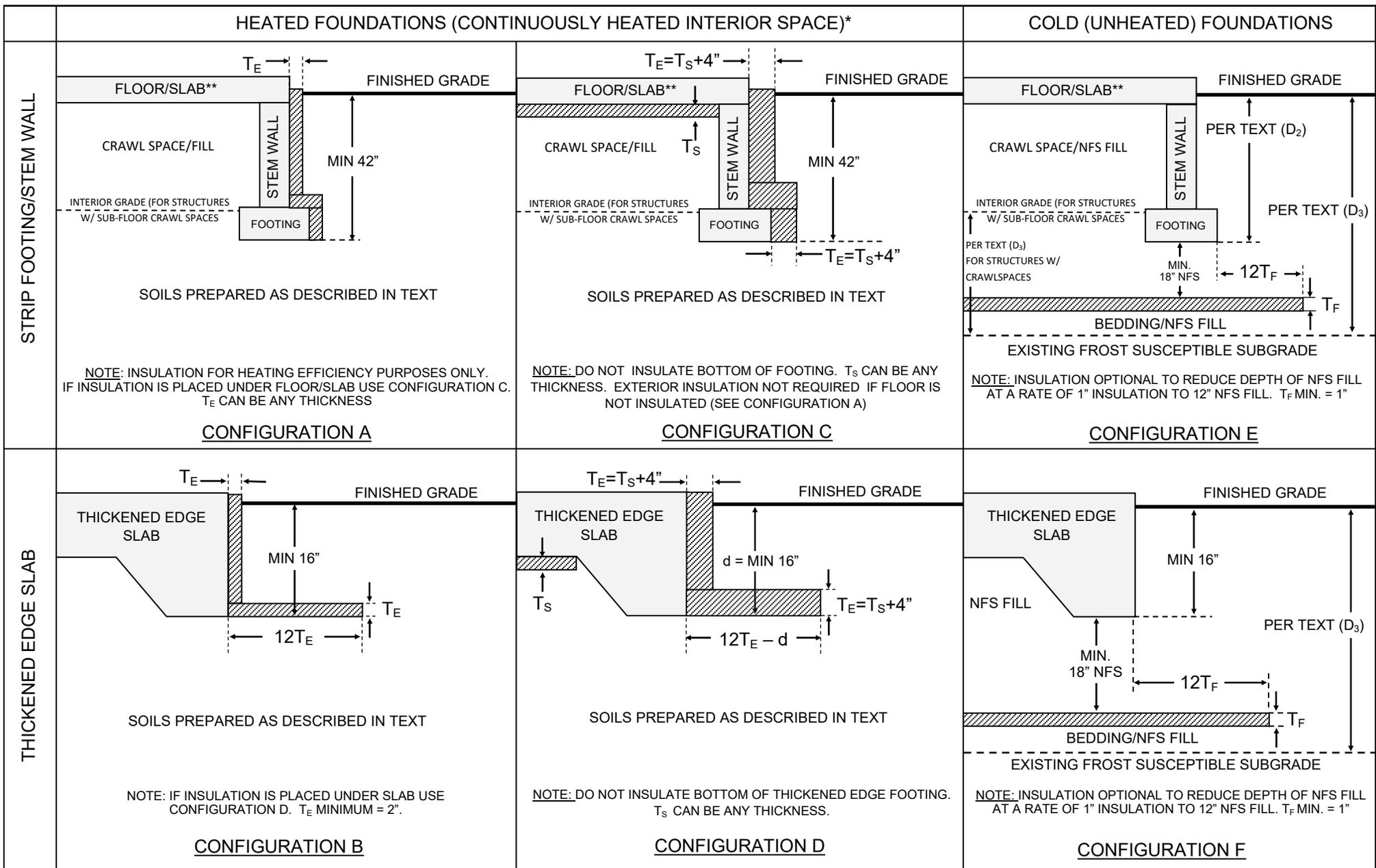
$T_F$  = INSULATION THICKNESS UNDER ENTIRE FOUNDATION (INCHES)
