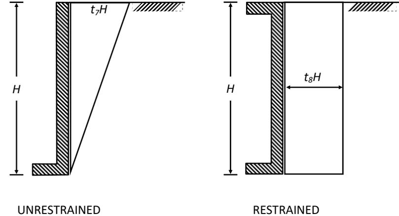
NOTE: WALLS CAN BE EITHER FREE OR RESTRAINED AT THE TOP FOR THE PASSIVE PRESSURE CONDITION. EQUATIONS ARE ONLY VALID FOR UNITS OF  $t_{1-8}$  (PCF) AND  $H-H_1$ (FT).
