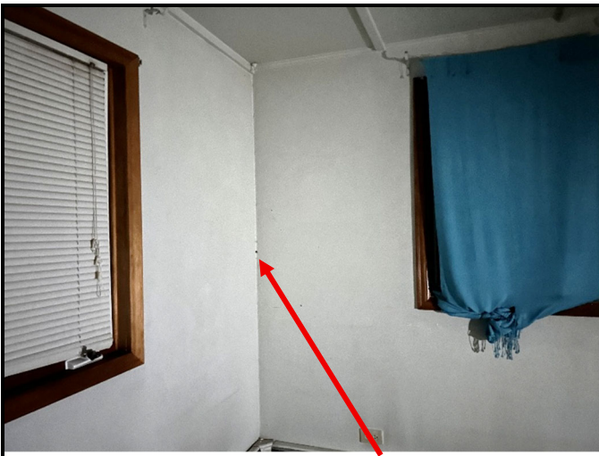
Photo 7. PACBM and PCBs sampling location, wall material in kitchen/living area – Sample AS10/PCB10
